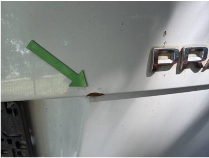
Heckklappe (Lackschaden, Rost)
