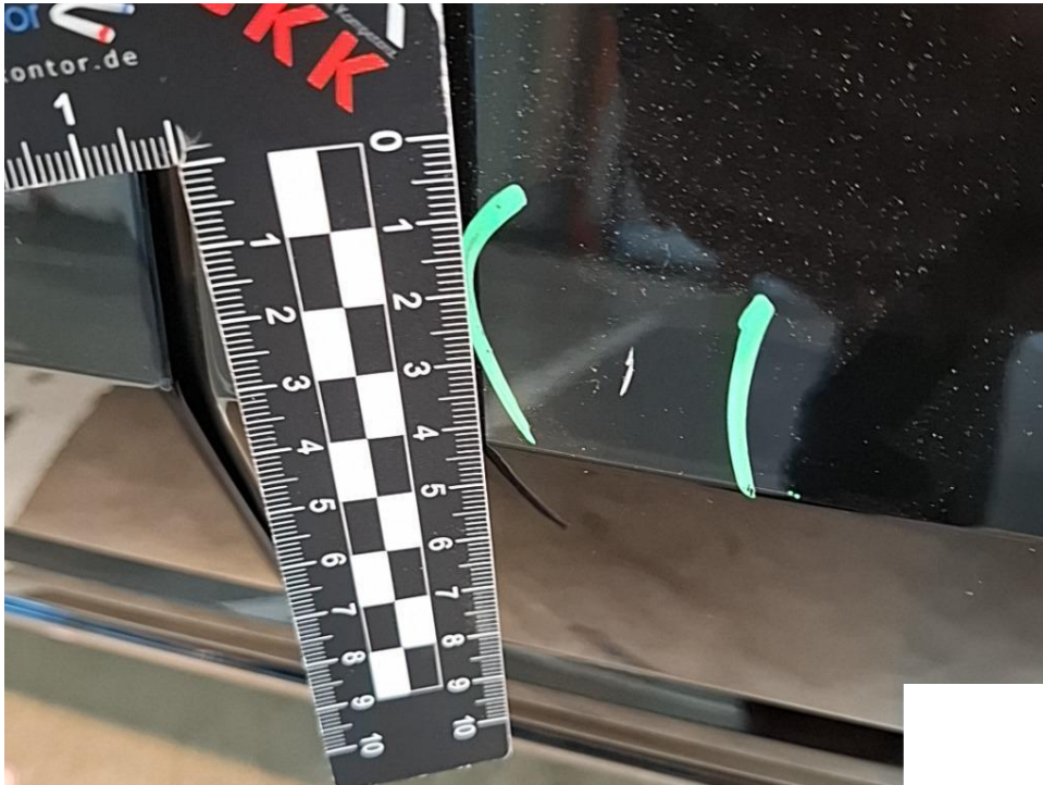
Picture 20 door rear left, scratched, disassemble, grind, polish
