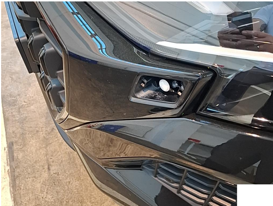
Picture 21 headlight cleaning system, cover, missing, replace
