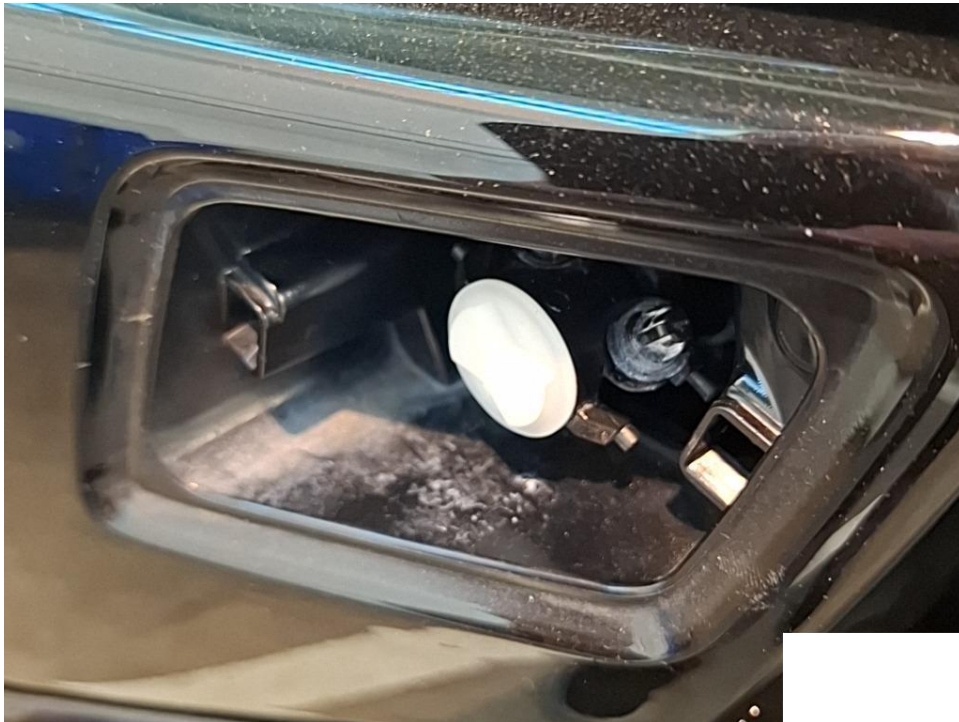
Picture 22 headlight cleaning system, cover, missing, replace
