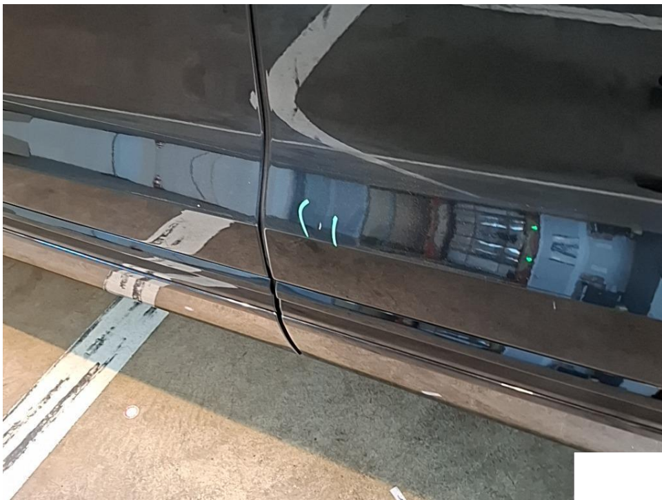
Picture 19 door rear left, scratched, disassemble, grind, polish
