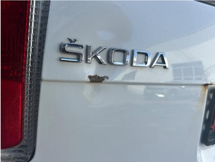
Heckklappe (Delle, Rost)
