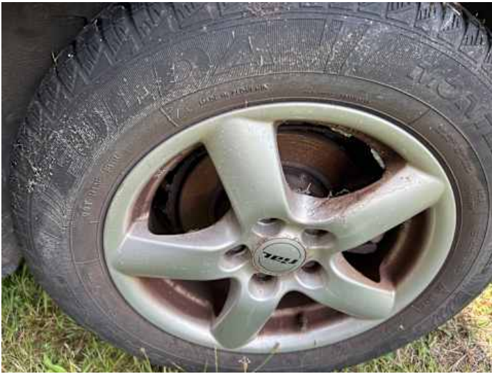
Rad (vehicle.damage-label.porous, Rost)
