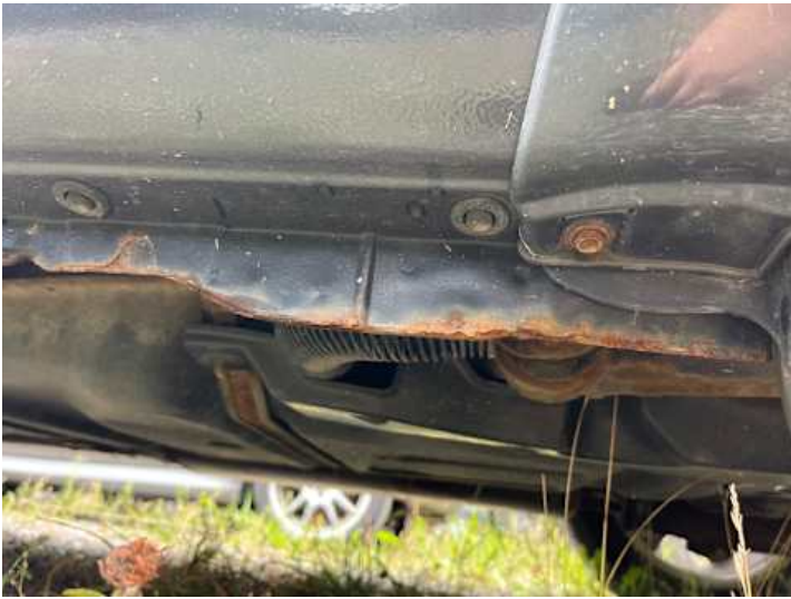
Schweller links (Lackschaden, Rost)
