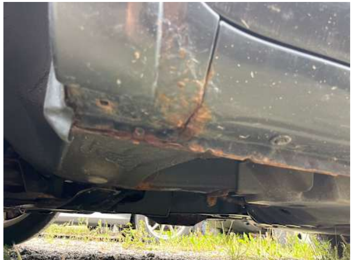
Schweller links (Lackschaden, Rost)
