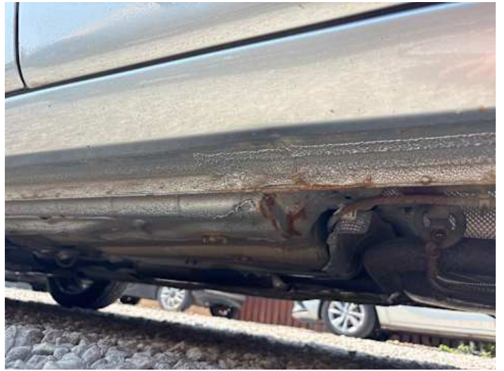
Schweller links (Lackschaden, Rost)
