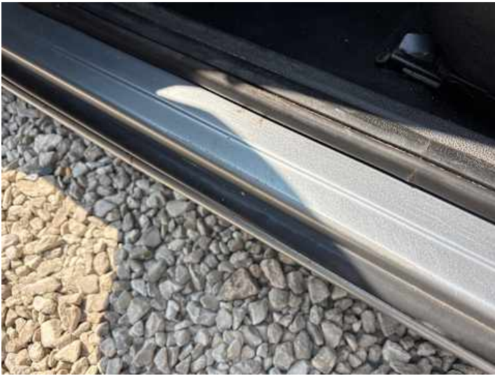
Schweller links (Lackschaden, Rost)
