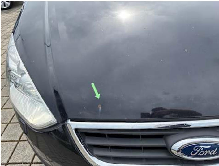
Motorhaube (Delle, Rost)
