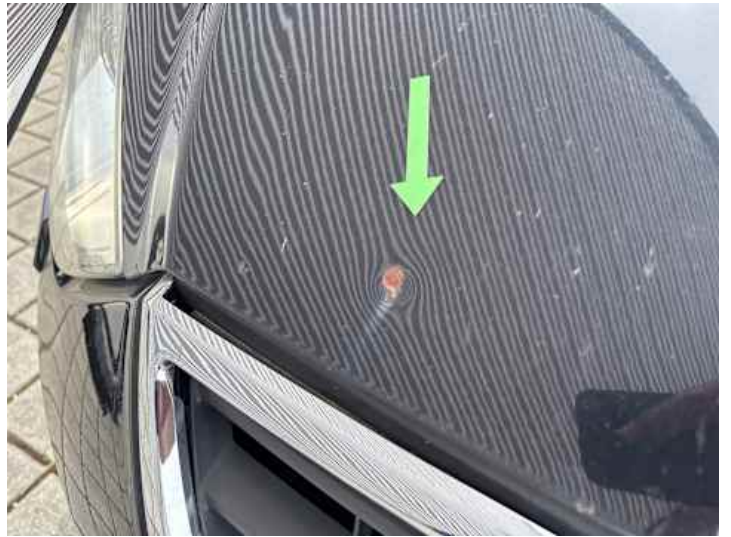
Motorhaube (Delle, Rost)
