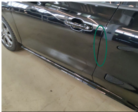
Tür / Vorne Links / Kratzer
