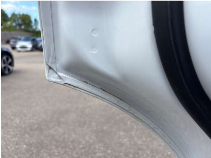
Türe hinten links (Lackschaden, Rost)
