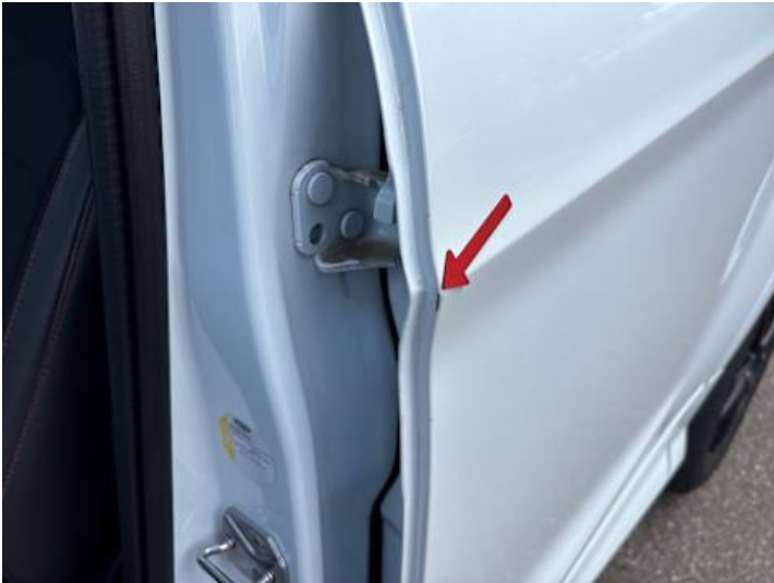
Türe hinten links (Lackschaden, Rost)
