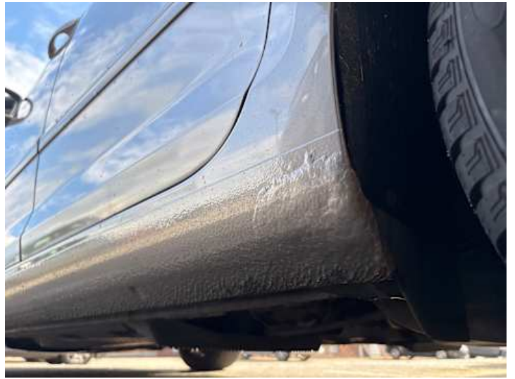
Schweller links (Lackschaden, Rost)
