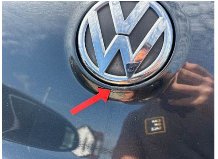
Heckklappe (Lackschaden, Rost)
