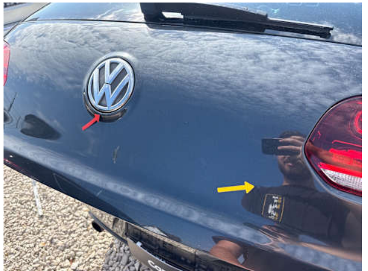
Heckklappe (Lackschaden, Rost)
