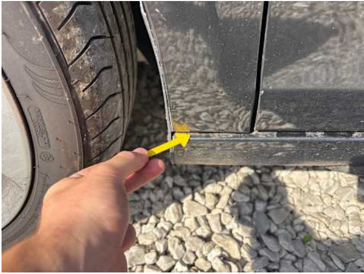
Schweller links (Lackschaden, Rost)
