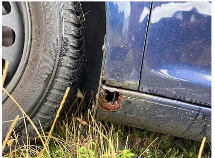
Schweller links (Riss/Bruch, Rost)
