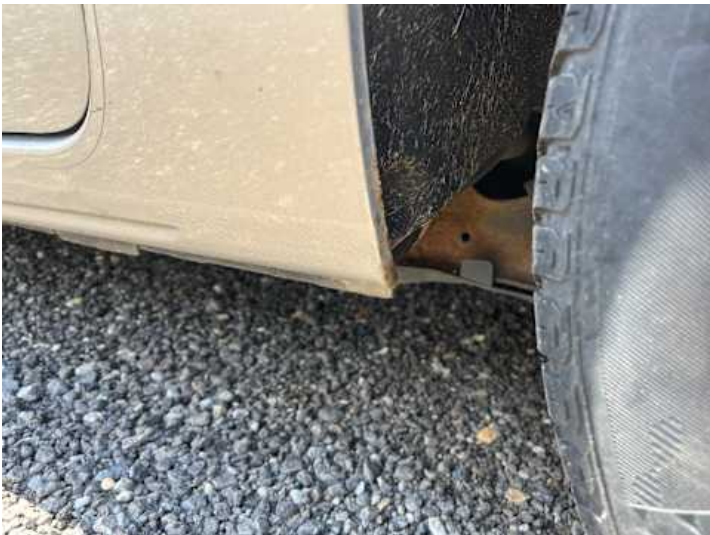
Schweller links (Lackschaden, Rost)
