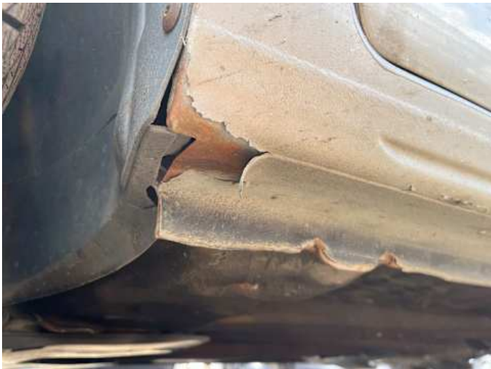
Schweller links (Lackschaden, Rost)
