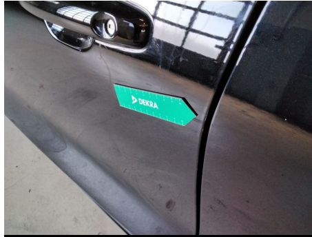
Tür / Vorne Links / Kratzer
