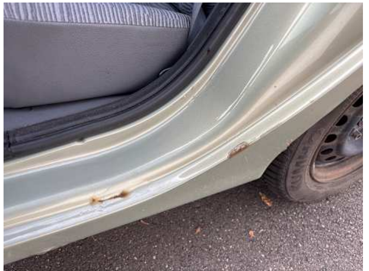
Schweller links (Lackschaden, Rost)
