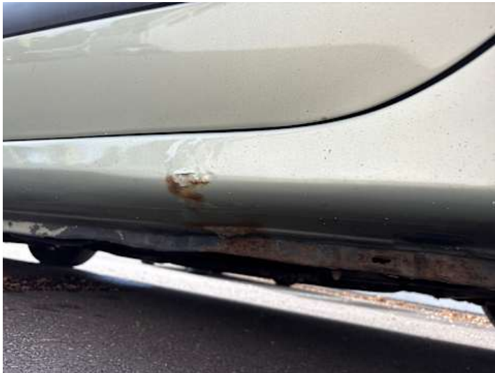
Schweller links (Lackschaden, Rost)
