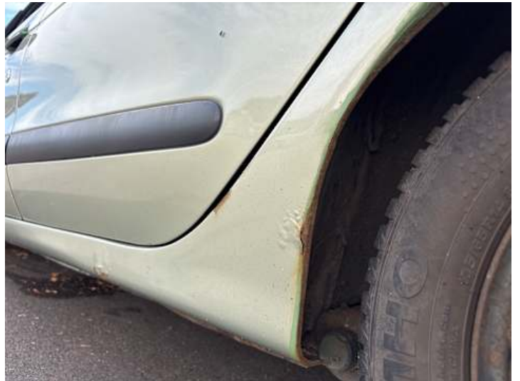
Schweller links (Lackschaden, Rost)
