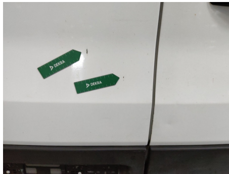
Heckklappe / Kofferraumtür / Hinten Links / Kratzer
