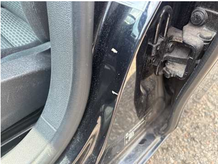
Schweller links (Lackschaden, Delle, Rost)
