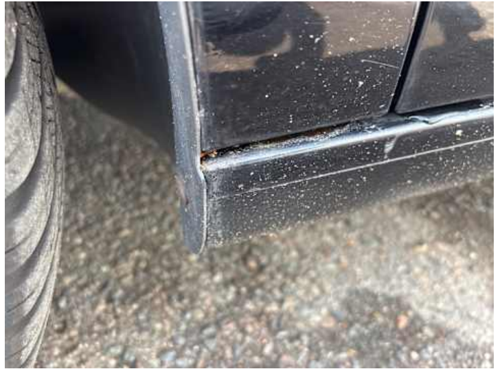
Schweller links (Lackschaden, Delle, Rost)
