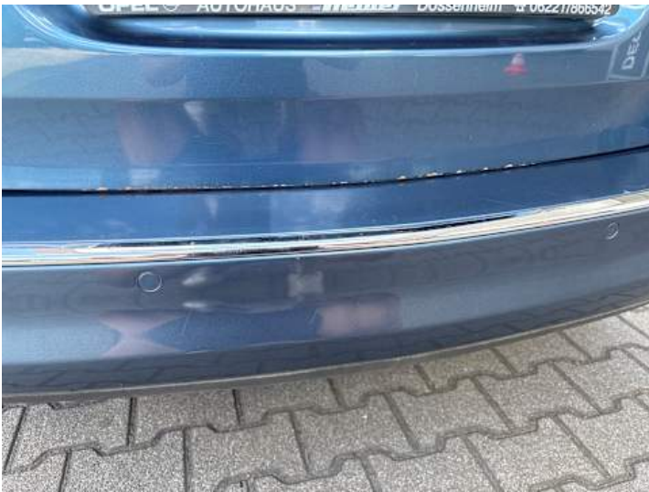
Heckklappe (Lackschaden, Rost)
