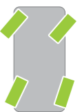
With rear-wheel steering: Front and rear wheels turn in the same direction
