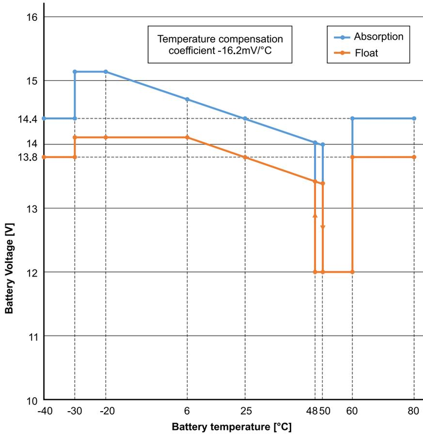
With a temperature sensor installed to the User I/O connection block; the actual battery temperature will be used for compensation; throughout the day.
