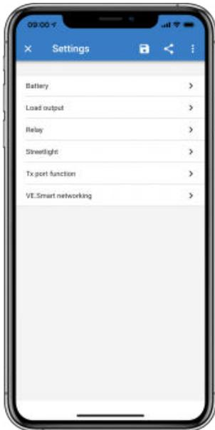
The settings page is accessed by clicking on the Cog icon at the top right of the Home page. The settings page provides access to view or change the settings of the Battery; Load; Streetlight; and Port functions. From this page you can also view Product information such as the Firmware versions installed on the MPPT Solar Charger.
