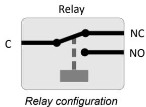
Use VictronConnect to check the relay functionality setting. When checking the relay check if the relay contacts are opened and closed when the relay is energized and also when the relay is not energized.
