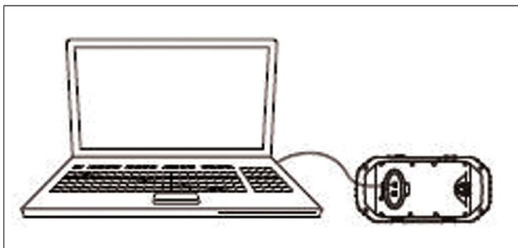
Charge the built-in battery by connecting the Poolboy to the PC via USB cable (included in the scope of delivery).
