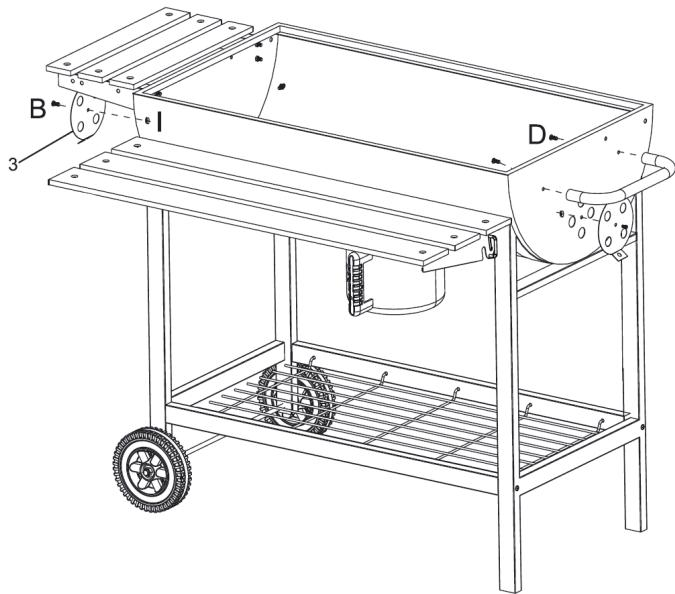
Attach the handle (1) to the side of the fire tray with 2 screws (D). Fasten the air vents (3) to the side of the fire tray with 2 screws (B) and 2 nuts (I).
