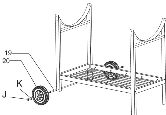
Insert the axle (19) through the holes of the short leg (14) and attach the wheels (20) to both sides of the axle. Attach the washer (K) to both ends of the axle and tighten with 2 M8 nuts (J).
