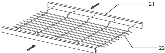
Insert the ends of the wire grate (22) into the matching holes of the metal brace (21).
