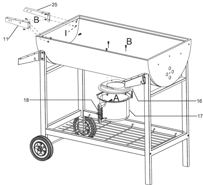
Fasten the connector of the ash container (16) to the bottom of the fire tray (6) using 3 screws (B) and 3 nuts (I). Fasten the bakelite handle to the ash container with 2 screws (A). Attach the ash container to the connector. Attach the supports for the side shelf (11 & 25) to the side of the fire tray using 4 screws (B) and 4 nuts (I).
