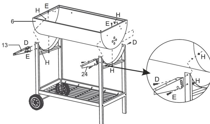
Attach the fire tray (6) and the front shelf support (13 & 24) to the legs using 4 screws (D), 4 pieces of bolts (E) and 8 M6 nuts (H).
