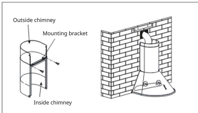
5. Adjust the height of the inside chimney to the position of the inside chimney bracket and fix on it by screw, meanwhile, fix the outside chimney on the cooker hood body by screws. See Pic 5. After adjusting the position, fix the body with safety screw.
