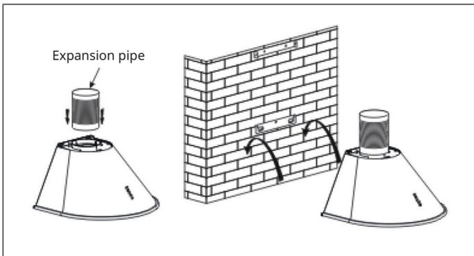
4. Fix the outside chimney bracket on the outside chimney, and be sure that the inside chimney can be adjusted the height in it freely. Afterwards, install the chimney on the cooker hood and lift up expansion pipe till it out of the wall through the hole on the wall.
