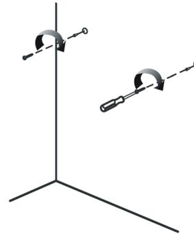
**NOTE:** You will need to ensure the screws are long enough to sufficiently grip the wall while allowing 5mm between screw head and wall.
