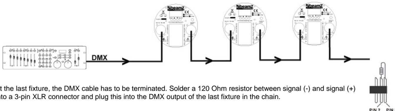
At the last fixture, the DMX cable has to be terminated. Solder a 120 Ohm resistor between signal (-) and signal (+) into a 3-pin XLR connector and plug this into the DMX output of the last fixture in the chain.
