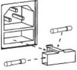
Step 1: Open the fuse holder on the rear panel with a fitting screwdriver.
