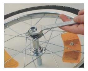
Remove the locknut and washer from the axle (9).
