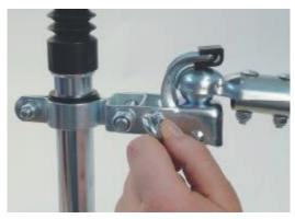
Tighten the securing screw in order to hold the coupling in place. This will prevent the ball-head coupling and tow bar becoming separated during use.
