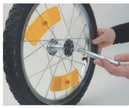
Insert the axle (9) through the hub of each 305 mm (16") wheel (3). Refit the washer to the axle (9), then tighten the locknut. Ensure that each locknut is correctly tightened. Check the locknuts at regular intervals for correct tightness.
