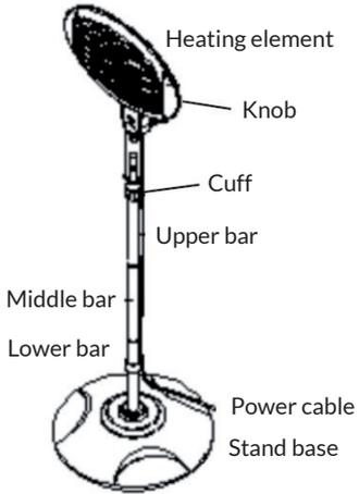
Connect the heating element (1) to the upper bar (7), tighten it by turning the knob. Pass the mains cable through the clamp.
