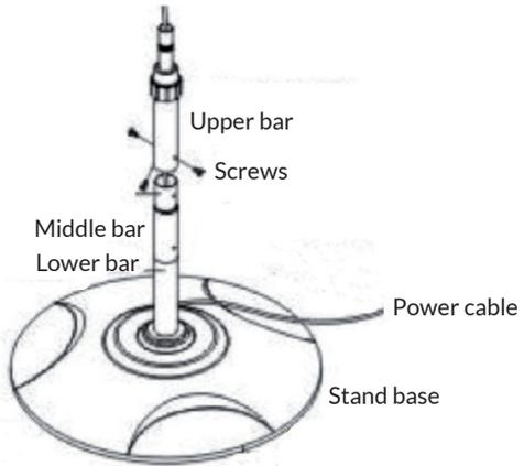
Insert the upper bar (7) onto the middle bar (9) and screw the bar together with a Phillips head screw.
