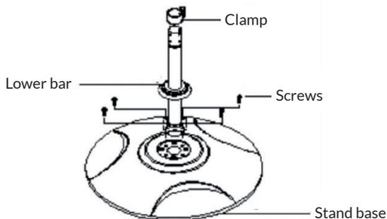
Insert the lower bar (11) into the stand (16) and tighten it with a Phillips screw.
