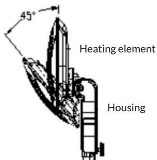
Depending on requirements, the angle of the heating element can be set to an angle of 0-45 degrees.
