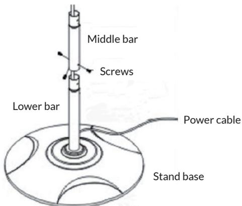
Insert the middle bar (9) into the lower bar (11) and fix the rod with a Phillips screw.
