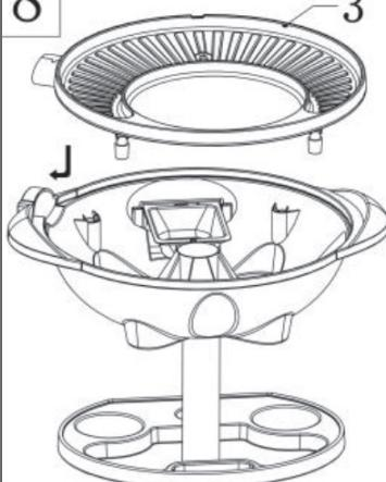
Put the fat collecting bowl (4) into the bracket supplied for it in the base of the appliance, buckle the hole of fat collecting bowl onto the screw to fix it well (The flat collecting bowl can be filled with little water to make it easier to clean).
