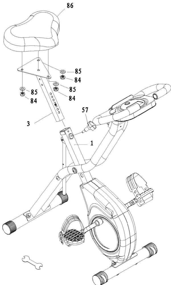
Mount the saddle (86) on the seat post (5) and secure the connection with 3 nylon nuts (84).
