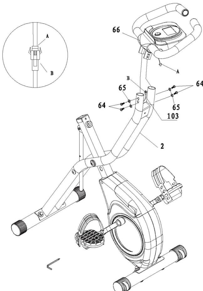
Mount the training computer on the front (2) and secure it with 4 allen screws (66) and appropriate washers (65).
