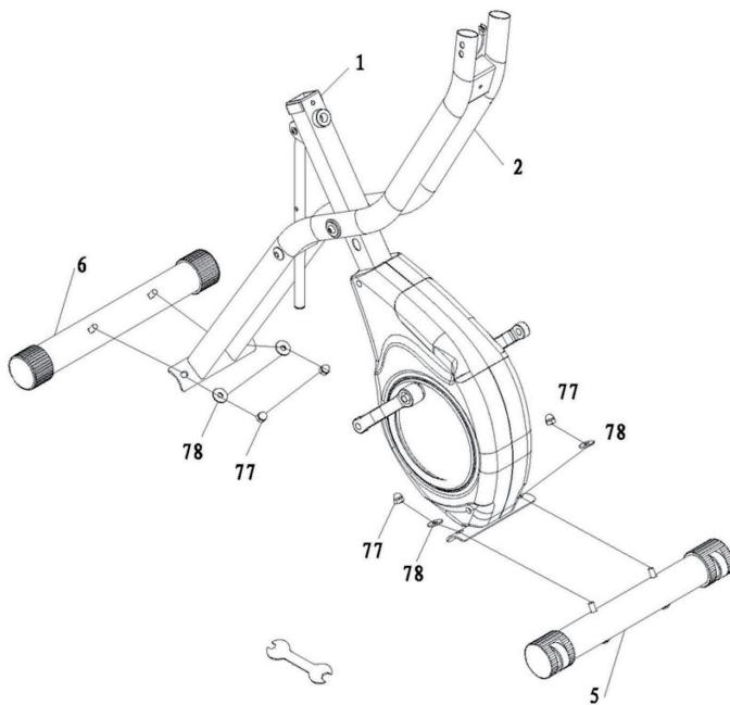
Mount the feet (5 & 6) on the frame (1). Use the domed washers (78) and the cap nuts (77).
