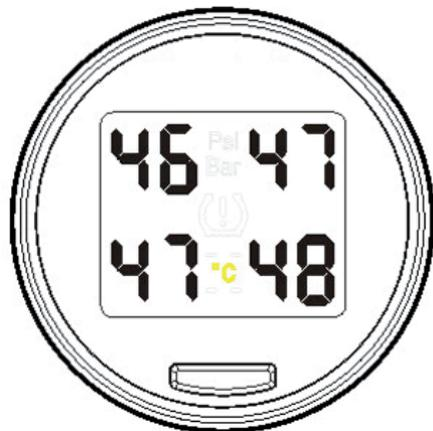
The display will show temperature unit °C if the tire temperature is above 0°C, and will show °C if it is under 0°C.
