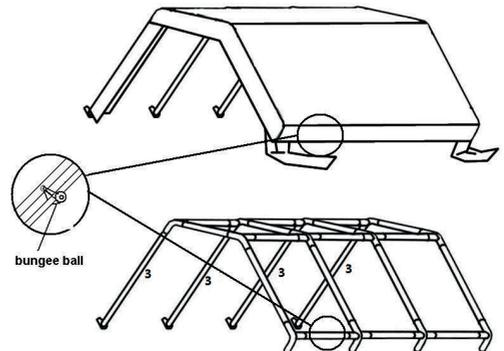
4. Attach the another 4 supported poles (3) to the joints (5,6), built-up the framework, use the 6x180 mm peg to fix each pole into the ground and use the hook to fix the leg cover to the ground.
