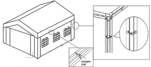
6. The guy lines clasp to each corner of tent and another end of line fix to ground by pegs (8x300 mm).
