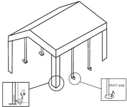
5. Spread the wall panel and door panel attach to framework by using the bungee cords clasping the frame to grommets that is construct over the wall panel and door panel to ensure stability. Also use the short pegs to fix the doors to the ground.
