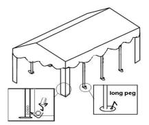
5. Spread the wall and door panels, and attach to framework using the bungee cords. Clasp the frame to the metal eyelets (located over the wall and door panels) to ensure stability. Also use the 4x180mm pegs to fix the doors and walls to the ground.
