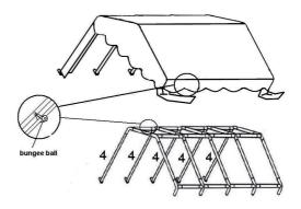
4. Attach the other 5 supporting poles (4) to the joints (6,7), build-up the framework .Use the 6x180mm peg to fix each pole into the ground and use the hook to fix the leg cover to the leg.
