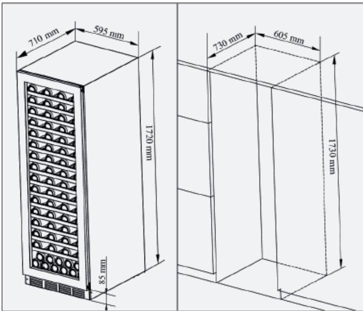
Unpack and remove all of the protection and adhesive strips from the packaging around and inside the wine cellar. The wine cellar must be positioned such that the plug is accessible. Release the power cord. Move your wine cellar to its final location. The wine cellar should be installed in a suitable place where the compressor will not be subject to physical contact.
