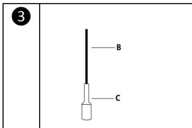
Insert the stick of the water-level indicator on the float.
