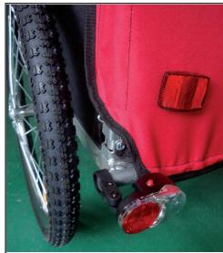
Insert the flagpole into the hole on the side and make it tight.
