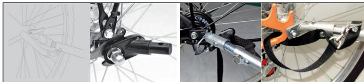
**Important:** The coupling between the bicycle and the trailer is the most important part of the assembly. Ensure that the trailer is securely coupled to the bicycle.
