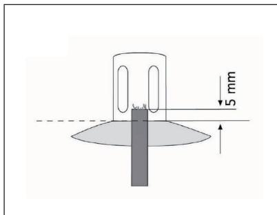
The wick opening must be completely tight. Due to the purely capillary effect of the wick supplied, it does not burn down and does not need to be replaced.
