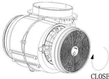
*Note: Make sure the filter is securely locked. Otherwise, it would loosen and cause dangerous. When activated carbon filter attached, the suction power will be lower.*
