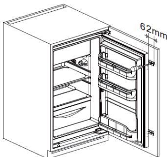
Slowly and carefully slide the unit into the cabinet. Make sure that the opening side is as close as possible to the cabinet wall and that the front is flush with the front of the built-in cabinet.
