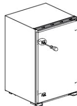
Remove the 4 screws from the front of the door. Then attach the two guides to the door with the 4 screws.
