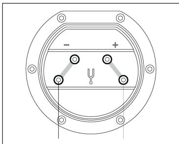
Then connect one end of your speaker cable to the two lower terminals of your speaker. Now, when connecting the other end to the amplifier, be sure to connect the PLUS terminal (usually RED) of the amplifier to the PLUS terminal of the connection panel - and MINUS (usually BLACK) to the MINUS.
