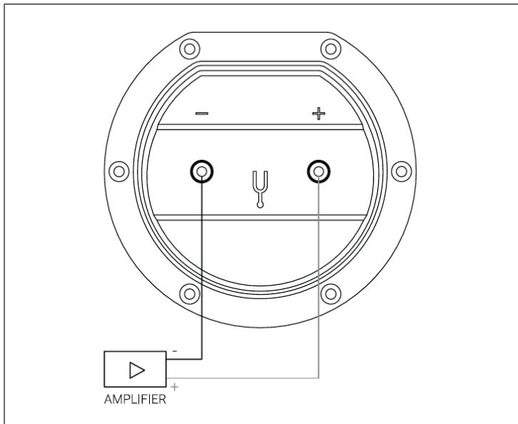
Please first connect one end of your cable to the two terminals on your speaker. Then when you connect the other end to the amplifier, please make sure to connect the PLUS terminal (usually RED) of the amplifier to the POSITIVE terminal of the connection panel - and NEGATIVE (usually BLACK) to NEGATIVE.
