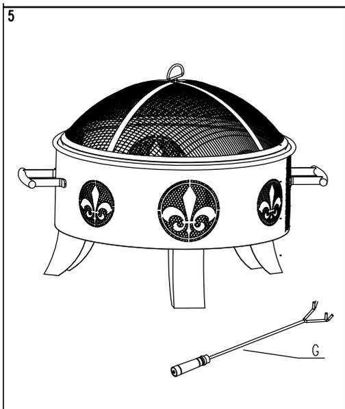
5. Take off the cover grid with the gripper arm.
