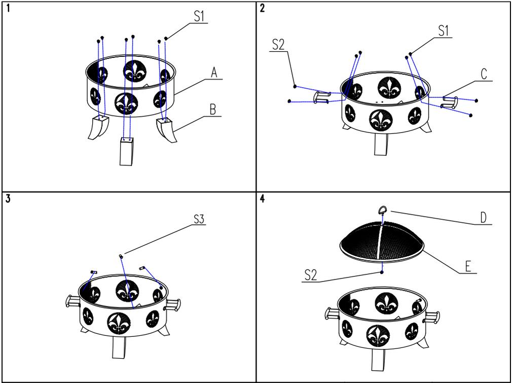
1. Position legs (B) and fix with screws (S1) to the bowl (A).
