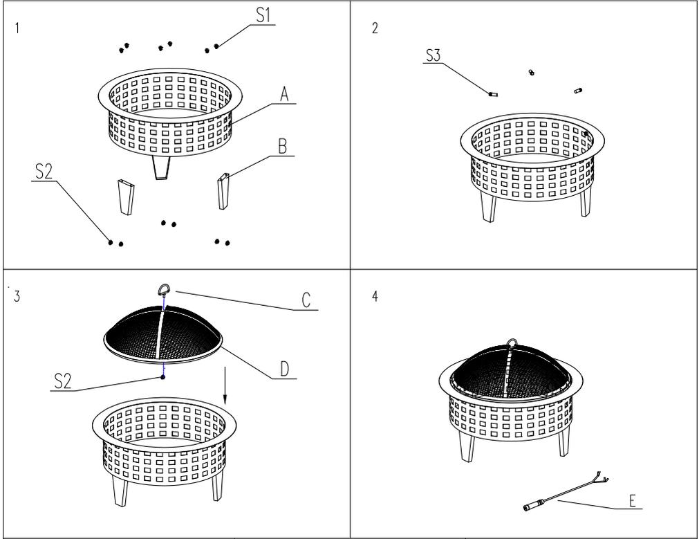
1. Position legs (B) and fix with screws (S1) to the bowl (A).
