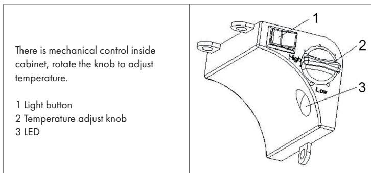
There is mechanical control inside cabinet, rotate the knob to adjust temperature.
