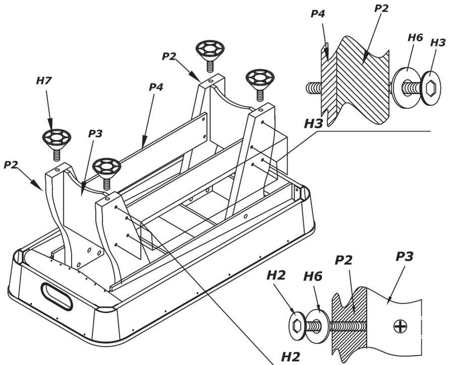
1. Attach the end leg panels (P3) to the inside surface of legs P2 using  $\frac{1}{4}$ " bolts H2 and washers (H6). (The threaded barrel are pre-assembled in the end leg panels P3).
