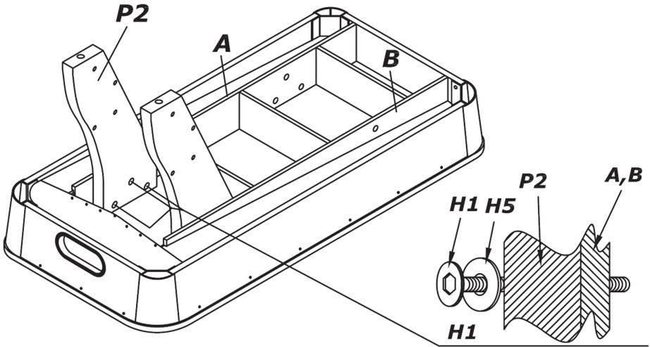
1. Place Main Assembly with the playing side on the ground. Take care the surface is even and clean. Underlay the shipping carton to avoid marks, scratches or other damage.
