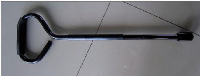
2. Place the assembly of the handle (15) and the connector (14) into the fork (13). Make the holes in the pull handle and the connector flush with each other. Insert M8x60 screws through the holes and tighten them with lock nuts (18).
