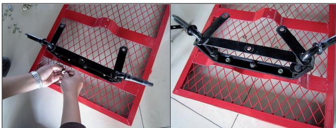
2. Place the fork (13) on the front axle bracket (10) by inserting the screws of the fork through the holes of the axle bracket (10)
