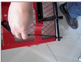
4. Align the holes on the flat ends of the left side of the rear axle guide (9) with the holes on the base (1). Insert the screws (16) from the bottom of the floor into the flush aligned holes. Place a washer (16) over the bolts and screw a nut (16) on top of each.
