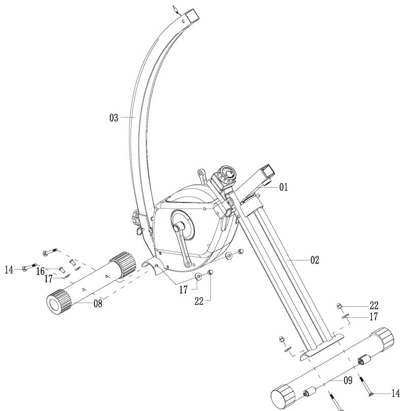
Attach the front stabilizer (8) to the main frame (1) and fasten it with two sets of carriage bolts (14), curved washers (17) and domed nuts (22). DO NOT FULLY TIGHTEN IT.
