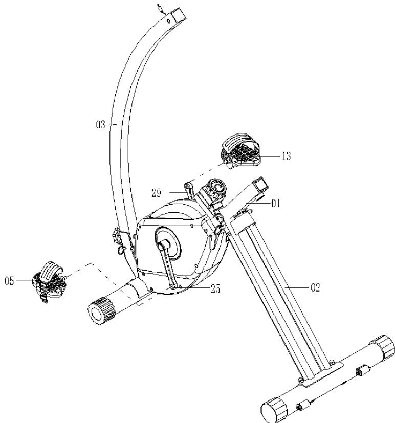
The left and right pedal (05) & (13) are marked „L“ and „R“. Connect them to their appropriate crank arm (25) & (29) of the main frame (1). The right pedal is on the right hand side of the cycle as you sit on it.
