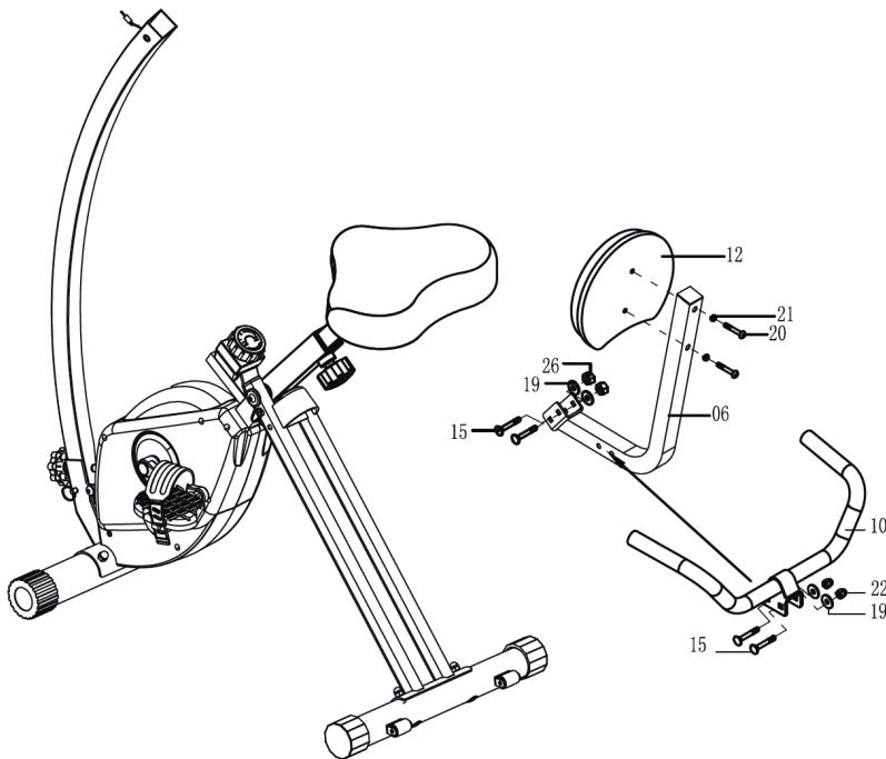
Attach the back support tube (6) to the seat support tube (4), tighten with two sets of carriage bolts (15), flat washers (19), nylon nuts (26).
