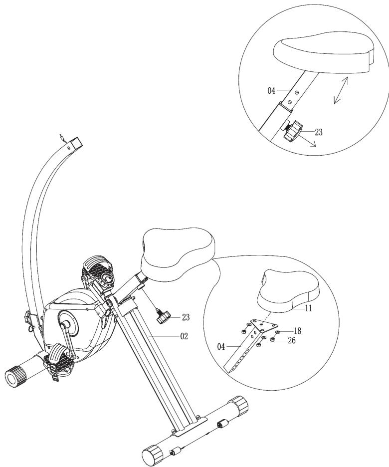
Take off three sets of nylon nuts (26) and flat washers (18) which are pre-assembled on the back of seat (11).
