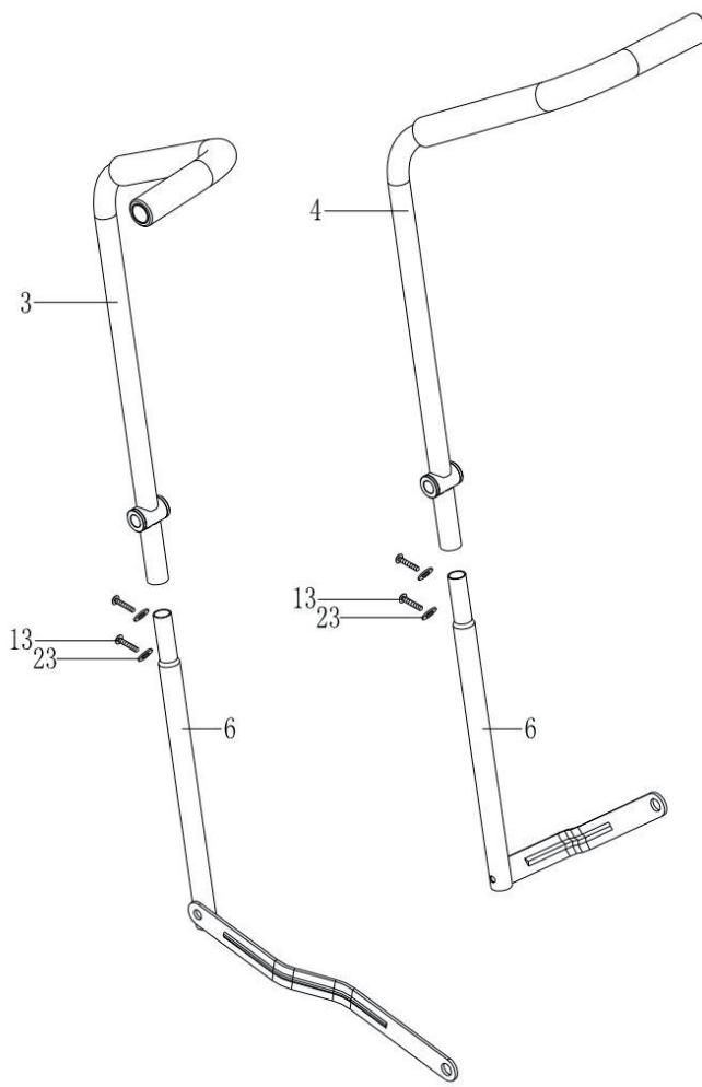
Put the upper and lower handle bar parts (3 / 4 and 6) together. Screw them together with two hexagon socket screws (13) and washers (23) each.
