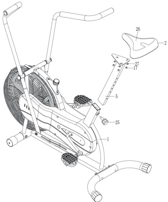
Remove the three nuts (27) and washers (27) from the saddle (26).
