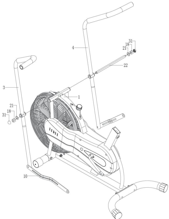
Remove the washer and plastic nut (21 + 18) from one side of the hub (22).
