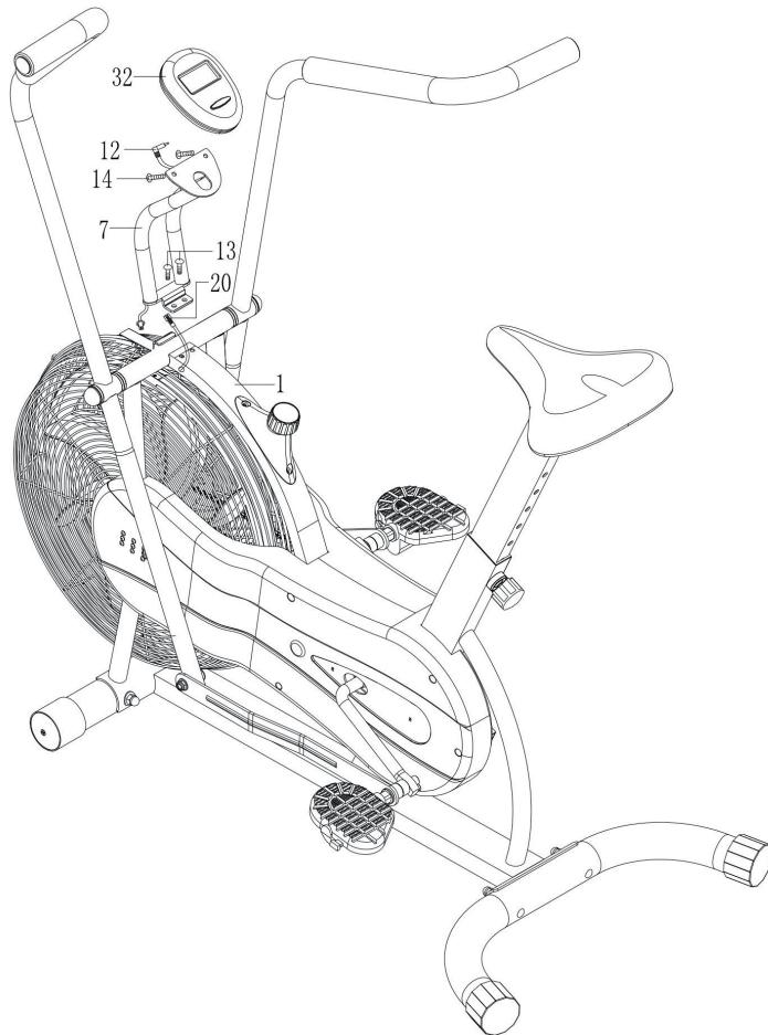
Join the two ends of the sensor cable (12 + 20) together.
