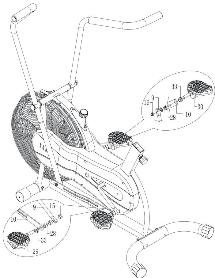
Remove the plastic nut (15) and the collars (33 + 28) from the left pedal (29).
