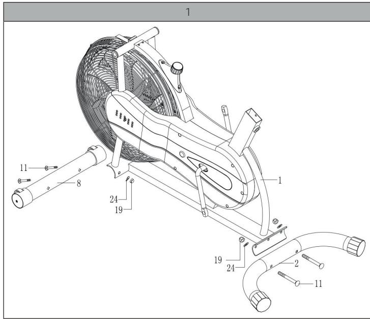
Mount the front foot (8) on the main part (1) and fix with two carriage bolts (11), two bow washers (24) and two cap nuts (19). Attach the rear foot (2) to the main body in the same way.
