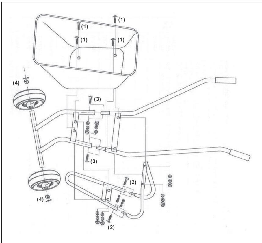
**Note:** Loosely tighten all screws at first during assembly. Tighten all screws at the end. It is recommended to assemble this wheelbarrow in pairs.
