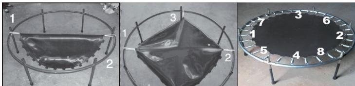
**Tip:** It is best to proceed in the manner shown here - connect opposite tabs to the frame in each case. This ensures that you do not skip any flaps and that the tension is built up evenly.
