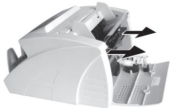
Disconnect the connector of the sensor.
