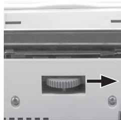
Retire the screws that hold the later cover. Retire the plate of the feeding deposit that extends down.
