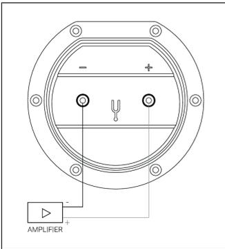
Please first connect one end of your cable to the two terminals on your speaker. Then when you connect the other end to the amplifier, please make sure to connect the PLUS terminal (usually RED) of the amplifier to the POSITIVE terminal of the Retrospective connection panel - and NEGATIVE (usually BLACK) to NEGATIVE.
